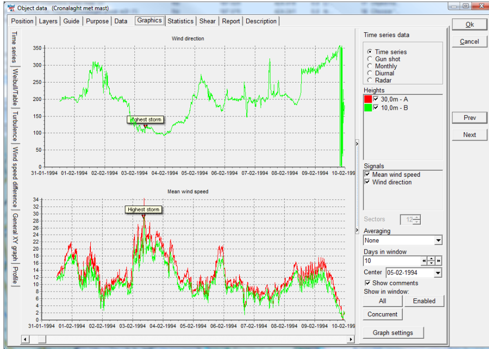
Figure 13 The time series view is efficient for finding erroneous data – simply right click in graph at start and end of erroneous data for disabling those. You can also add comments (right click) and these can be reported in a separate report.
