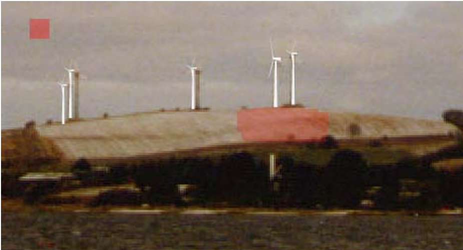
Figure 5 The rubber tool simply "paint" the rubber areas, where you do not want rendering. In that way you can rub a whole hill so even though you slightly move the turbines to be rendered behind the hill, there will be no visible parts in front of the hill.
