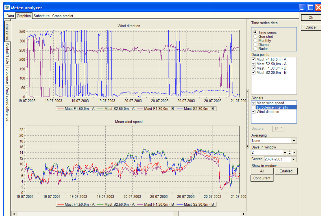
Figure 28 In the "graphics" tab, you will see basically the same graphs as in Meteo object, only now with comparison of data from more Meteo data objects.
