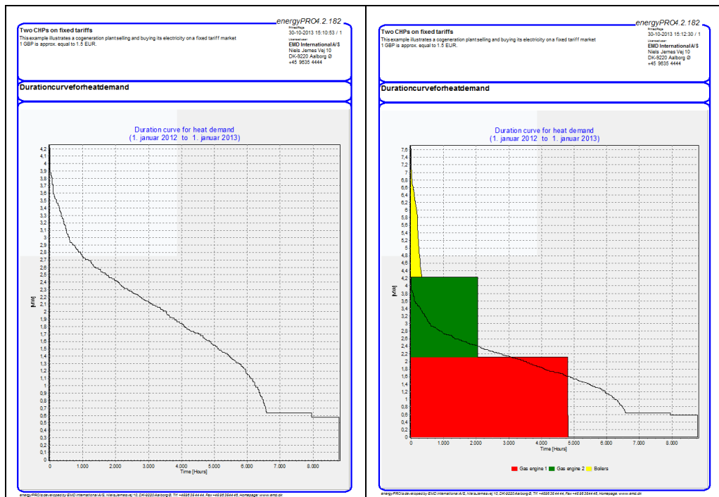
Figure 2.173: Duration curve for heat demand (left). Demand curve for heat demand with productions included (right)
