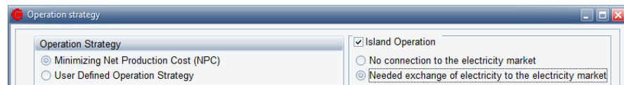
Figure 2.121: The island operation mode is visible in the upper right corner of the Operation Strategy when you have electricity demands in your project
