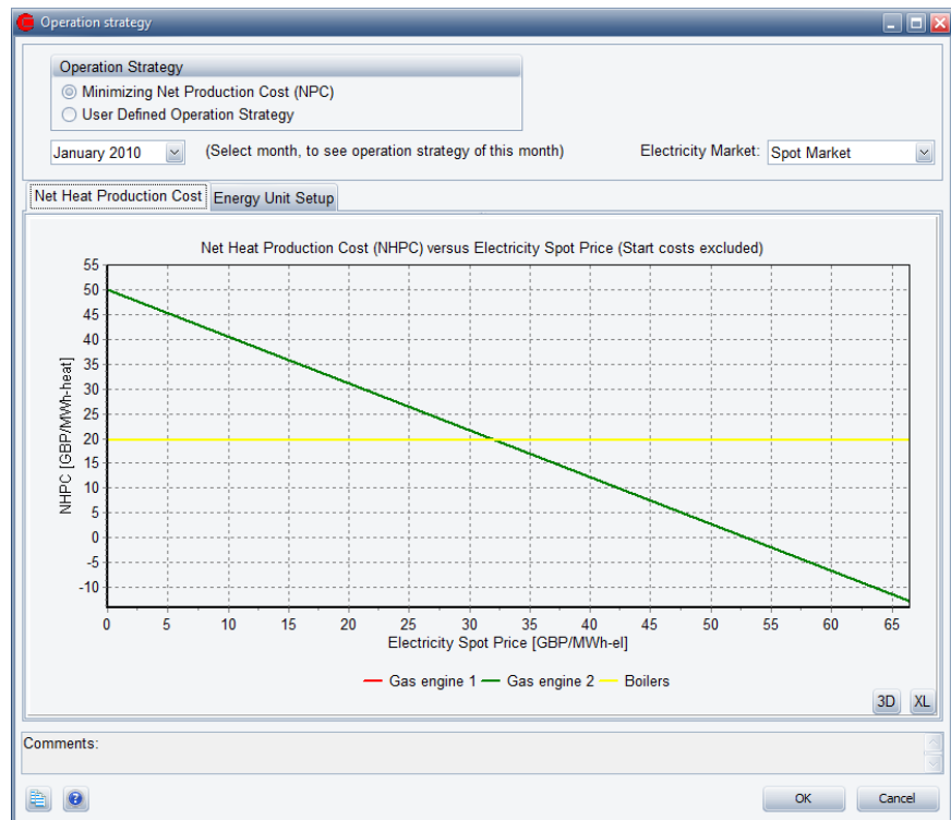
Figure 2.115: Operation Strategy window – Upper simple user defined example – lower auto calculated operation strategy example
