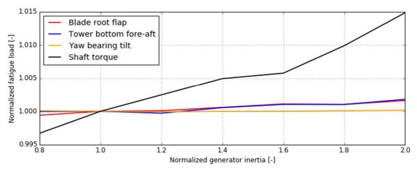
Figure 5: Fatigue load sensitivity to generator inertia normalized with respect to the default inertia of 250.000 kgm<sup>2</sup> for easy comparison.
