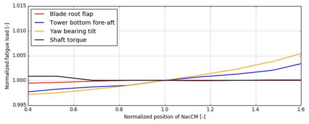
**Figure 6**: Fatigue load sensitivity towards the downwind position of NacCM normalized with respect to the default position of 1.9m downwind for easy comparison.
