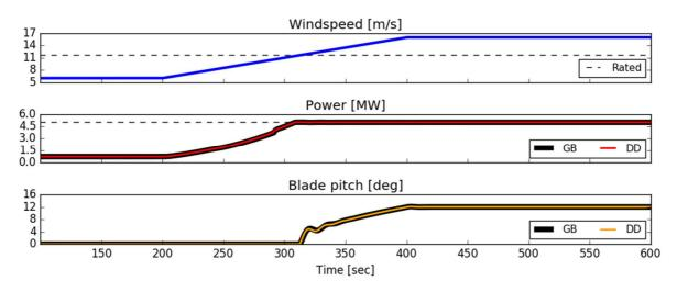
Figure 2: Comparison of the original and scaled controller during a linear increase in windspeed from 6m/s to 16m/s. GB is the original geared turbine and DD is the direct-drive version.
