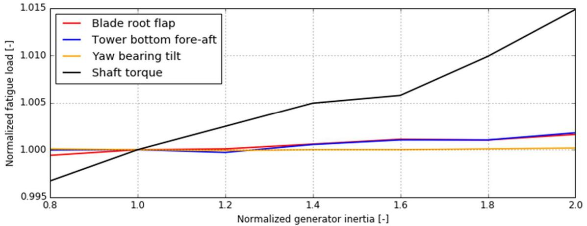
**Figure 5:** Fatigue load sensitivity to generator inertia normalized with respect to the default inertia of 250,000 kgm<sup>2</sup> for easy comparison.
