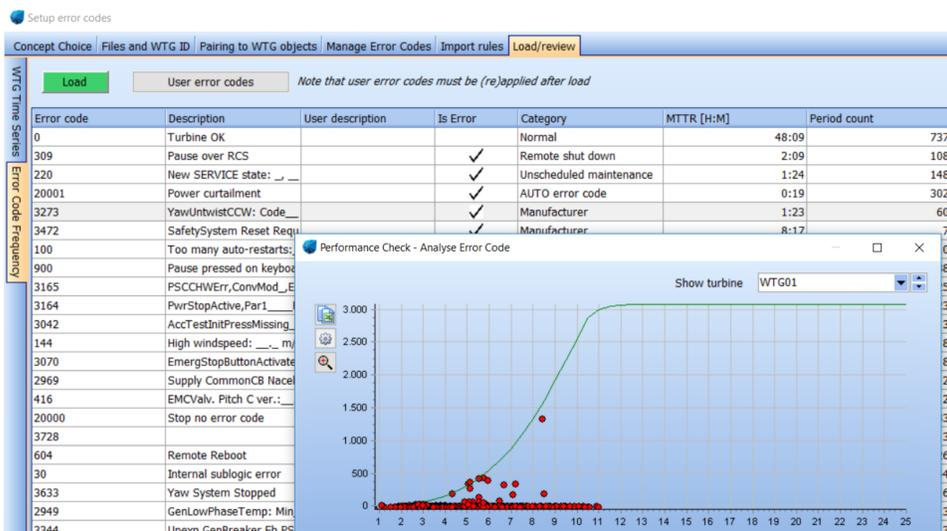
As example the above figure highlights events with an error code of 3273. This code represents all the events connected to cable CCW-untwist.
